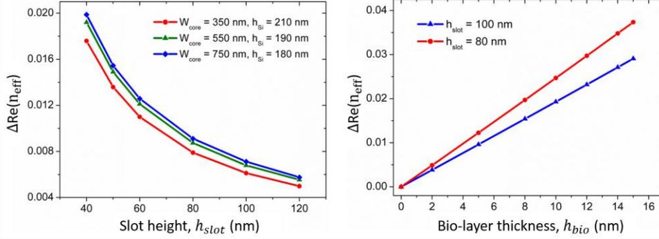
Fig. 3. (a) Real effective index difference [ $\Delta Re(n_{eff})$ ] variations due to ssDNA and dsDNA with slot height for optimized  $h_{Si}$  and  $W_{core}$ , depicts the CPWG sensitivity and (b) denotes the  $\Delta Re(n_{eff})$  variations with bio-layer ( $n = 1.45$ ) thickness for 80 and 100 nm slot height.
