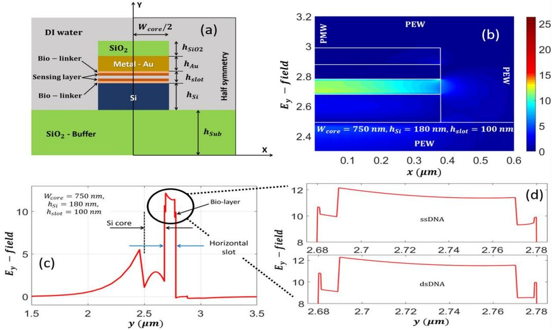
Fig. 1. (a) Schematic cross-section of the CPWG to detect DNA hybridization. (b)  $E_y$  field profile of half symmetric CPWG, (c) depicts the variation of  $E_y$  field along the y-axis symmetry line and (d) denotes the light confinement variations due to presence of ssDNA and dsDNA.
