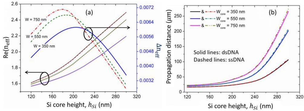
Fig. 2. Variation of  $Re(n_{eff})$  and propagation distance ( $L_p$ ) with Si core height for three different core widths,  $W_{core} = 350, 550$  and  $750$  nm
